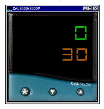
Note: the instrument display will show LEV5 if no valid setting has been made for input sensor, display resolution or output device, these settings are configurable from instrument front panel only.
