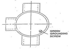
**WARNING!** For personal safety, this cabinet must be properly **grounded.** The ground wire to the cabinet must be installed on the green screw located in the conduit outlet box.
