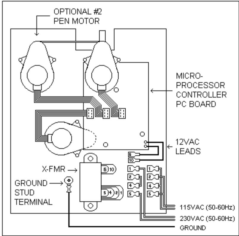
**Figure 6C:** Recorder Assembly Type "B" (Rear View).
