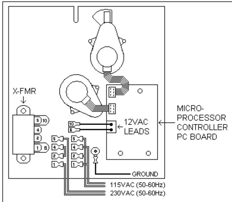
**Figure 6D:** Recorder Assembly Type "C" (Rear View).
