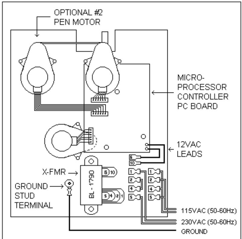
**Figure 6A:** Recorder Assembly "Type A" (Rear View).
