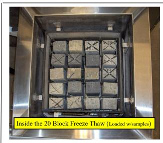
Our models hold from twenty (20) to eighty (80) 3" x 4" x 16" concrete test beams. However, specimen racks and cabinets can be customized to accommodate your needs.
